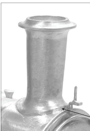
Note how the solder seem at the casting base is blended into the brass boiler.
